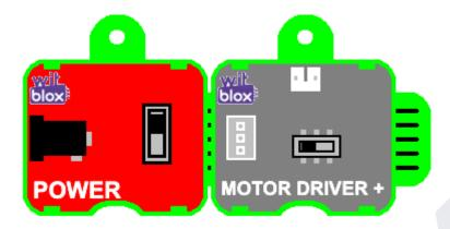
5. Lastly, flip the Power Switch on the Power Blox to ON and the mechanism should start working. The BO Motor combined with the geared link to lift up and pull down the parking lot barrier as needed.
